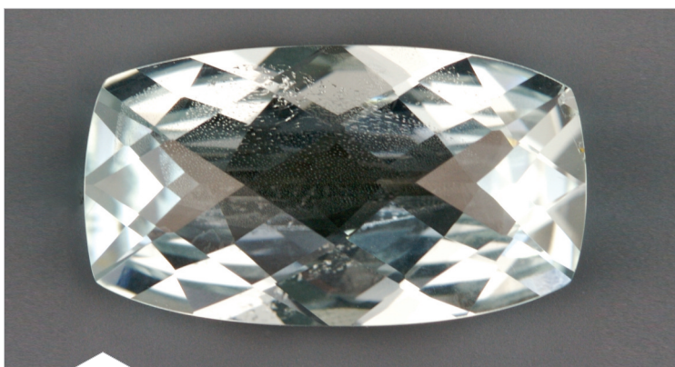
FIGURE 10. Aquamarine, precision cut, but with a large window.
